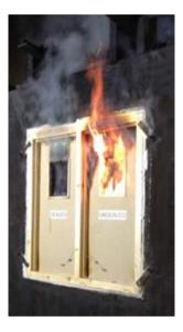
An example of a sealed vs. unsealed door during a fire threat.
